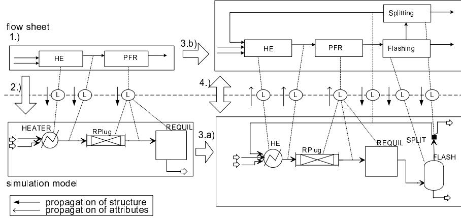
Fig. 1. Integration between flow sheet and simulation model
